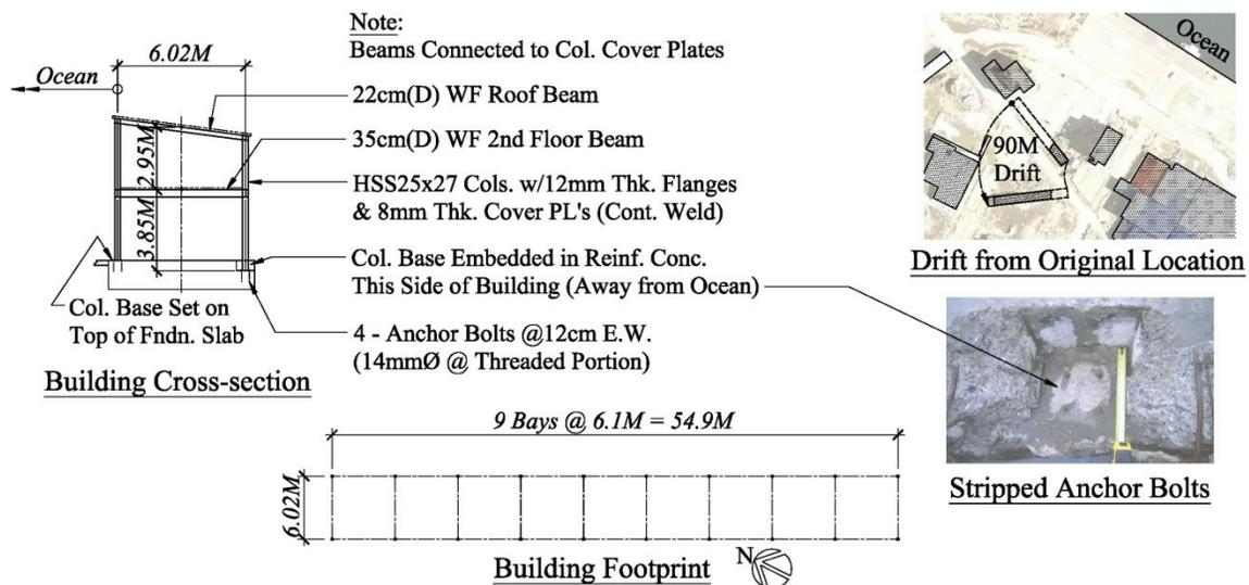
Figure 4. Lateral translation of entire warehouse building and failure of anchor bolts.
