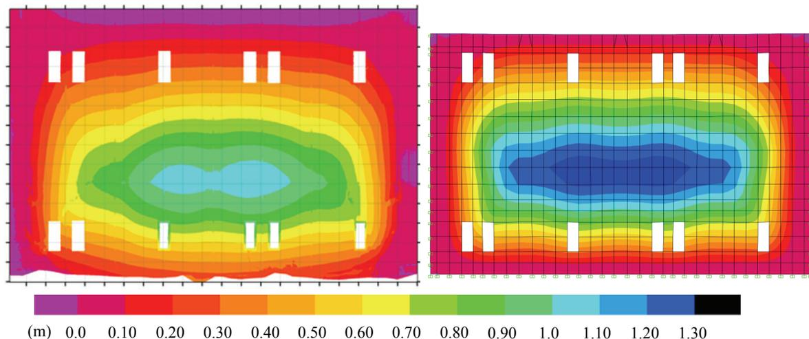
Figure 10. Deformation modeling using a triangulated LIDAR scan showing out-of-plane deformation (left) compared to a FEM analysis of damaged wall (right).
