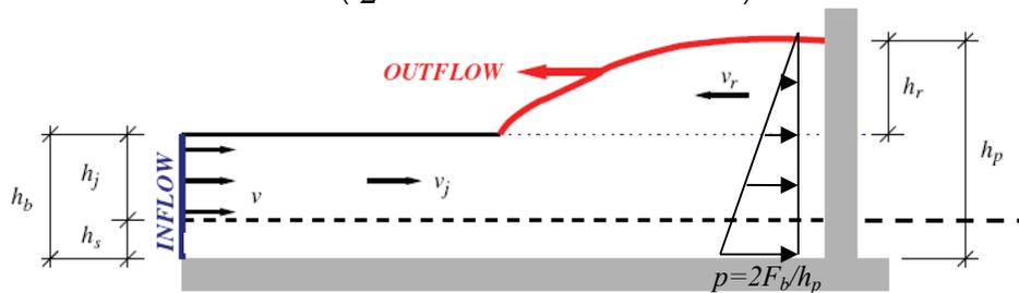
Figure 1. Tsunami bore travelling over standing water and striking a wall
