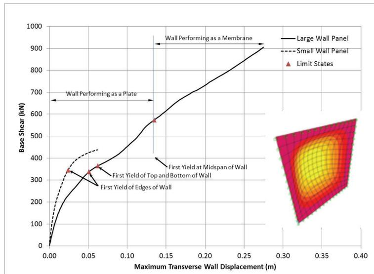
Figure 6. Total applied force versus maximum displacement of the wall and corresponding limit states for large and small wall panels.
