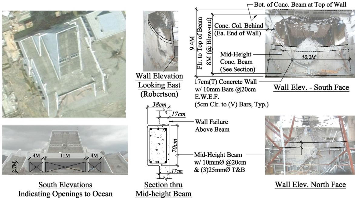
Figure 7. Large wall failure in the Takada Matsubara building in Rikuzentakata
