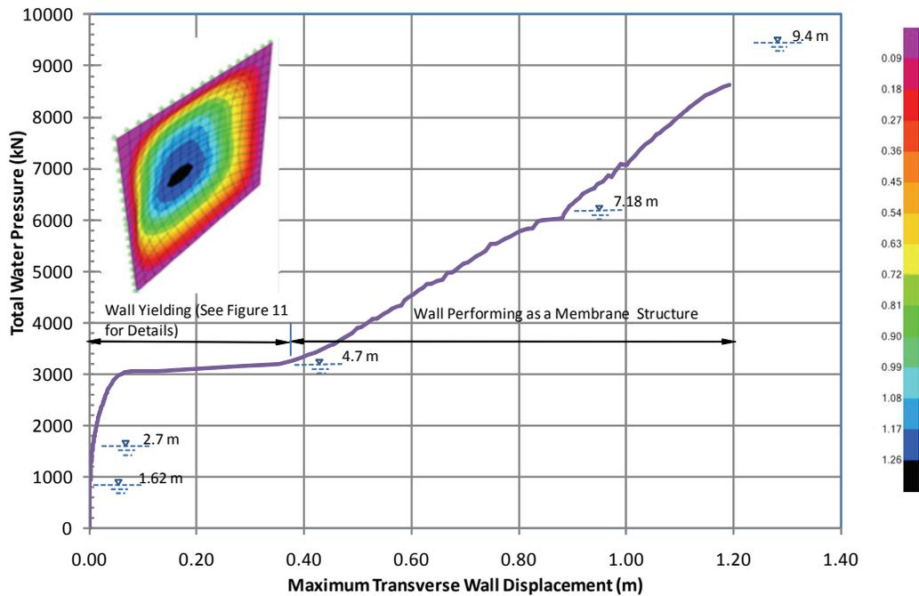
Figure 8. Load history of the total applied force versus maximum displacement of the wall
