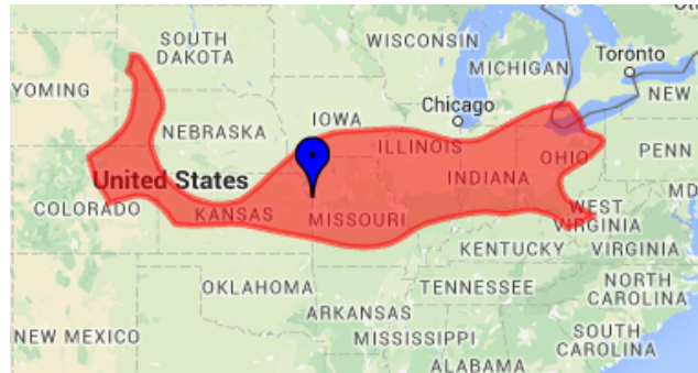
Ground Snow Load website image showing Kansas City located within a mapped area having a ground snow load of 20 psf.
