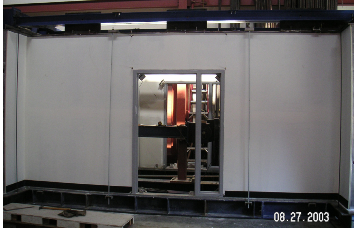
Figure 6. Testing of gypsum board partitions to develop fragility functions (after J. Restrepo and A. Filiatrault)
