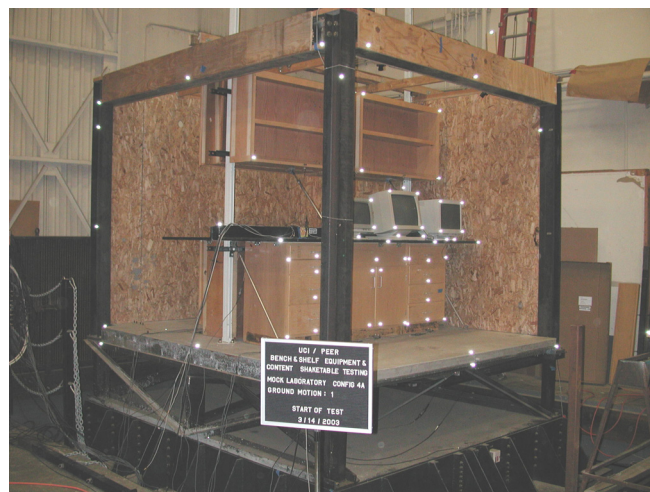
Figure 7. Testing of bench and shelf-mounted equipment (after T. Hutchinson)
